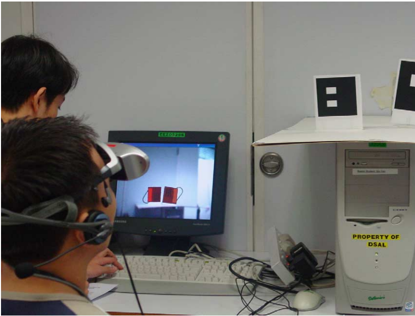
Fig. 4. The physical set-up of the experiment on depth judgment. The output of the computer VGA signal is sent to a monitor and HMD for display by a video converter. The user can only see from HMD while the monitor is for the use of the experimentalist. Two virtual telephones with different colors are augmented onto different markers respectively. The size of augmented objects is adjusted to about the same by adjusting the position of marker. Users are required to tell the relative depth of the two objects in the cases of with and without 3D sound aided.
