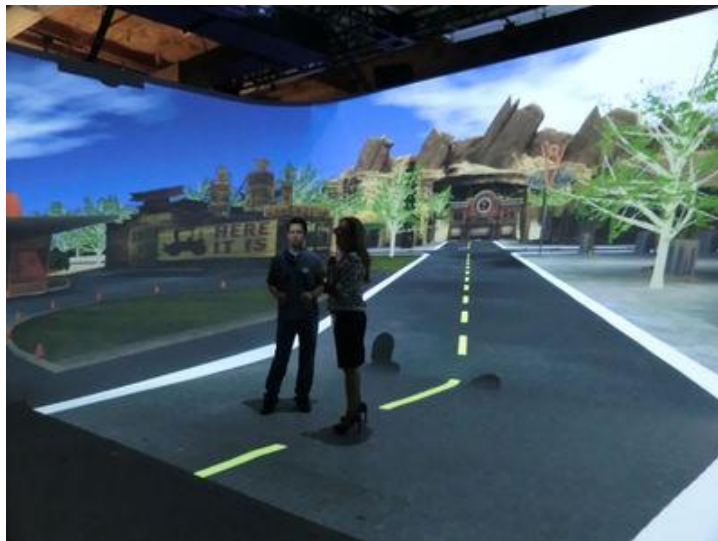
The DISH uses four projectors to create an interactive 3D environment. Photo by Adrienne Vincent-Phoenix.
