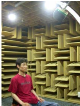
Figure 8: Experimental setup for the measurement of individual HRIRs in an anechoic chamber.
