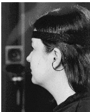
Figure 5. Microphones are placed near the entrance of the ear canal in a blocked-meatus position. The tracker sensor is held to the head via a Velcro strap.
