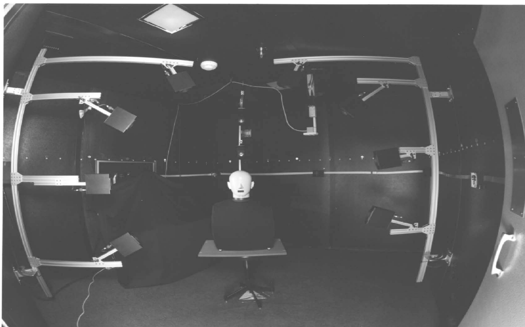
Figure 3. Fisheye lens view of loudspeakers within booth. Transmitter and microphone inputs are mounted on a wooden pole descending from the ceiling at the upper right of the head; aiming devices (section 1.5) are distributed at eye height.
