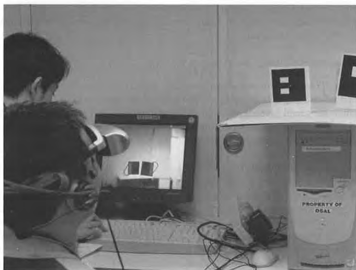
Fig. 4. The physical set-up of the experiment on depth judgment. The output of the computer VGA signal is sent to a monitor and HMD for display by a video converter. The user can only see from HMD while the monitor is for the use of the experimentalist. Two virtual telephones with different colors are augmented onto different markers respectively. The size of augmented objects is adjusted to about the same by adjusting the position of marker. Users are required to tell the relative depth of the two objects in the cases of with and without 3D sound aided.
