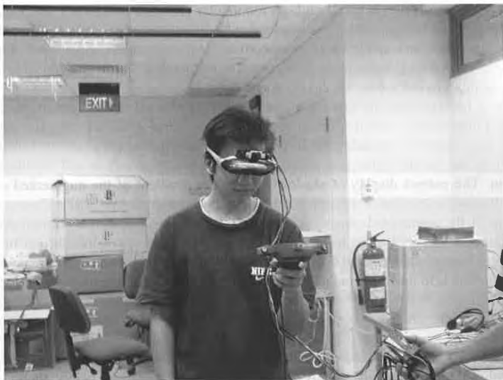
Fig. 3. The physical set-up of our acoustic-inertial tracking AR environment. On the ceiling there are six IS-900 SoniStrips which makes up a three meter by three meter area. A head tracker is mounted on the user's HMD and a camera is fixed on the head tracker. A wand tracker with four buttons and one joystick was held in the user's hand as an interaction device.
