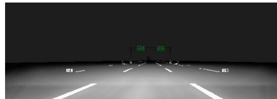
Fig. 10A The ISO diagram of test results of the LED fog lamp Fig. 10B Road render of test results of the LED fog lamp
