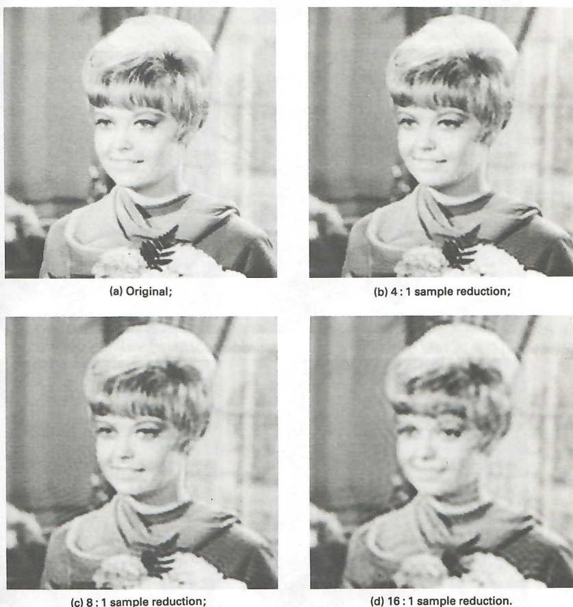
Figure 5.21 Basis restriction zonal filtered images in cosine transform domain.
