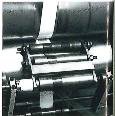
Ribbon cable production machine – copper conductors are sandwiched between insulating ribbons.
