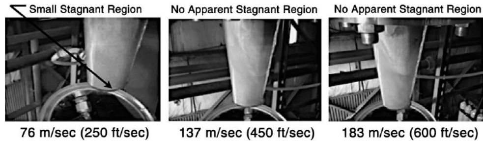
Fig. 17. Still shots from a video of the 3.8-cm (1.5-in.) bottom ID by 7.6-cm (3-in.) top ID conical jet cup with 100 g of material.
