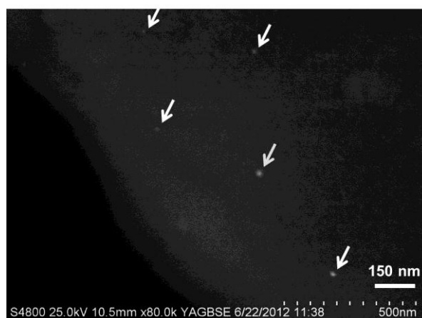
FIG. 2. YAG electron backscattering image and size distribution data from the deactivation sample in FCC unit after at least a thousand cycles. The average particle size is 13 nm which indicates a significant sintering which certainly will cause the degradation of the COP additives.
