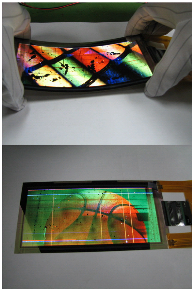
Figure 7. New top-emitting full-color OLED display on a stainless steel foil substrate
