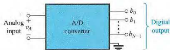
Fig. 1.9 Block-diagram representation of the analog-to-digital converter (ADC).
