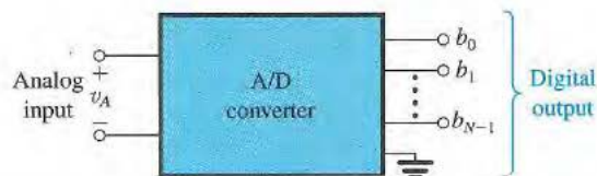
Fig. 1.9 Block-diagram representation of the analog-to-digital converter (ADC).
