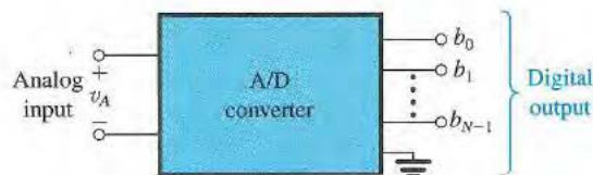
Fig. 1.9 Block-diagram representation of the analog-to-digital converter (ADC).
