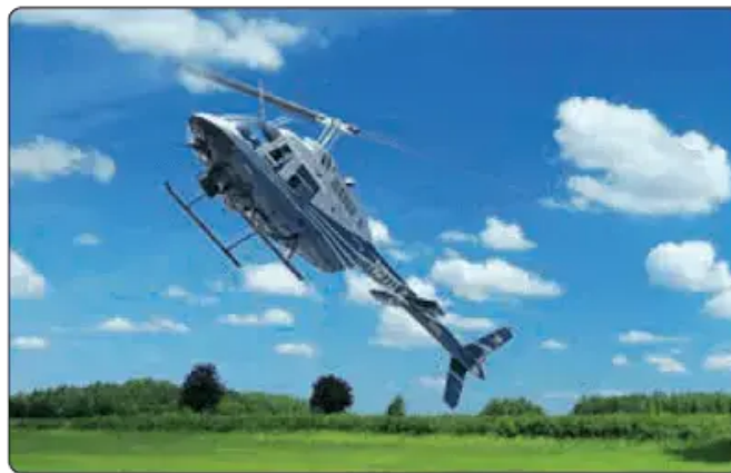
Figure 16. Bell Jet Ranger in final stage of autorotation
