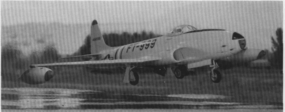
Figure 2.1.11. The first production U.S. jet fighter was the Lockheed P-80, powered by a single 2,000-pound engine developing approximately 4,000 pounds of thrust.
