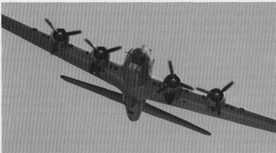
Figure 2.1.4. The B-17 Flying Fortress was powered by four Wright R-1820-97 nine-cylinder, air-cooled radial engines, which each delivered 1,200 horsepower. (Photograph by Barry Santana)
