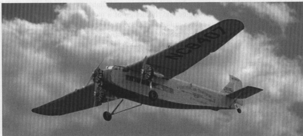
Figure 2.1.3. This 1929 Ford Tri-motor was powered by three J-5C Wright Whirlwind radial piston engines that each weighed 500 pounds and developed 220 horsepower, producing a power-to-weight ratio of 0.44 hp/lb. (Photograph by Barry Santana)
