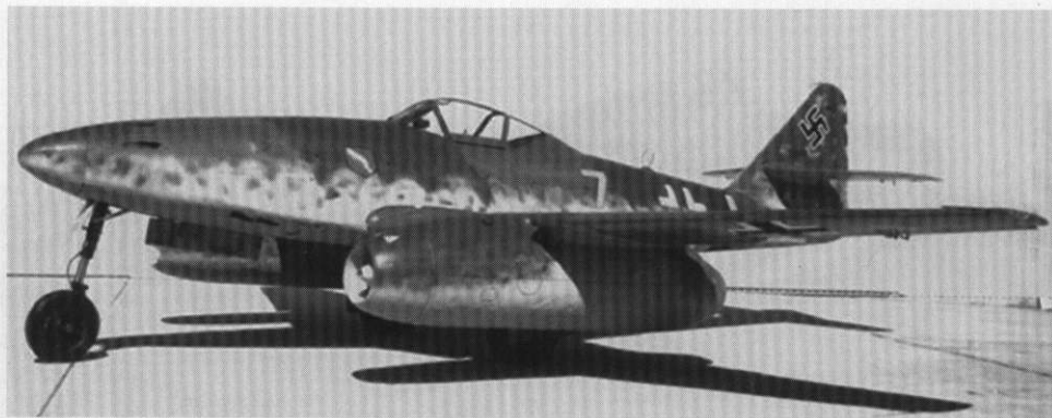
Figure 2.1.7. The first mass-produced jet fighter, the Messerschmitt Me-262, was powered by two turbojet engines, each weighing 1,650 pounds and developing 2,000 pounds of thrust. (Photo by Dale Hrabak, National Air and Space Museum, Smithsonian Institution, SI 79-4620)
