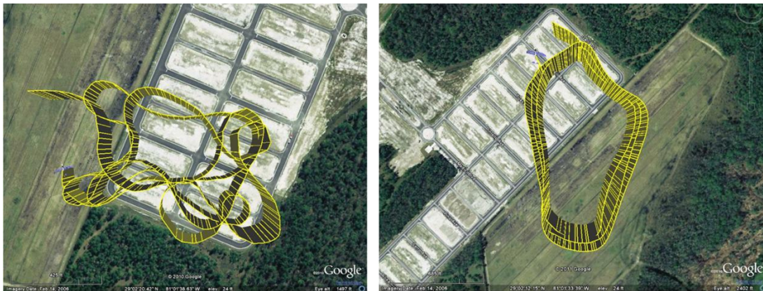
Figure 11 - Untuned Autopilot (Left), Waypoint Tracking after Tuning (Right)
