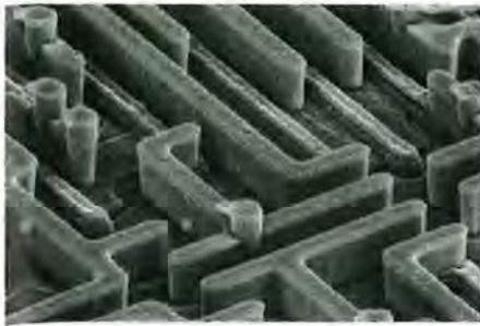
SEM Micrograph of Polysilicon, Tungsten LI and Tungsten Plugs (Polysilicon is represented by the thin lines between the taller LI lines). (Micrograph courtesy of Integrated Circuit Engineering)
