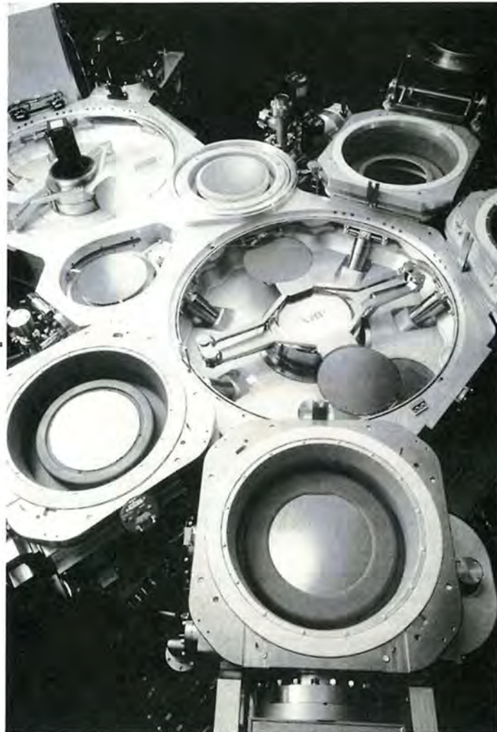
PVD Cluster Tool (Photo courtesy of Applied Materials, Inc.)
