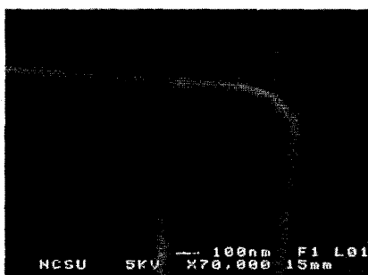
Figure 2: SEM image illustrating selectivity of SiGe deposition with respect to thermal oxide.
