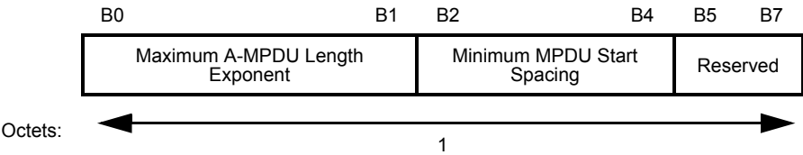
Figure 7-95o19—A-MPDU Parameters field
