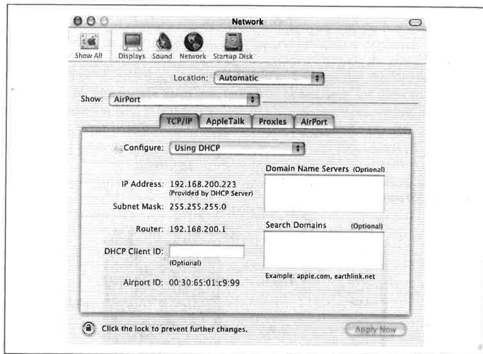
Figure B-7. TCP/IP preferences tab of the Network Preferences settings
