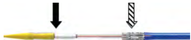
Fig. 4. The NovaFlex™ delivery system with the valve (striped arrow) crimped proximal to the inflatable balloon (black arrow) catheter.
