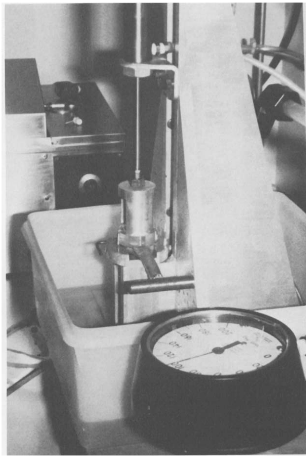
Fig 1. Porosity testing device. Graft material is fixed and sealed by pneumatic head. Water flow is adjusted by calibrated flowmeter until pressure is stable.
