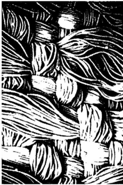
Figure 3a. SEM micrograph of woven double velour: face.
