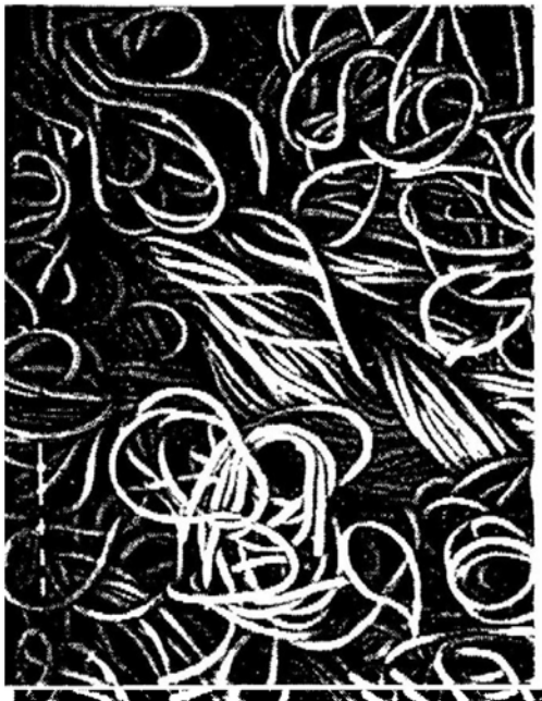
Figure 9b. SEM micrograph of Cooley double velour: back.
