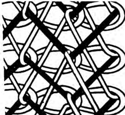
Figure 8. Reverse locknit structure.
