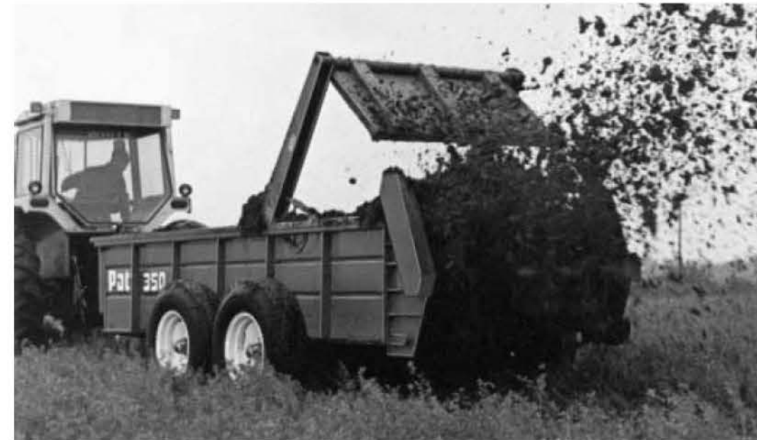
Figure 2. This box-type spreader is equipped with a chain-driven conveyor to move solid manure to the beaters for rear discharge.
