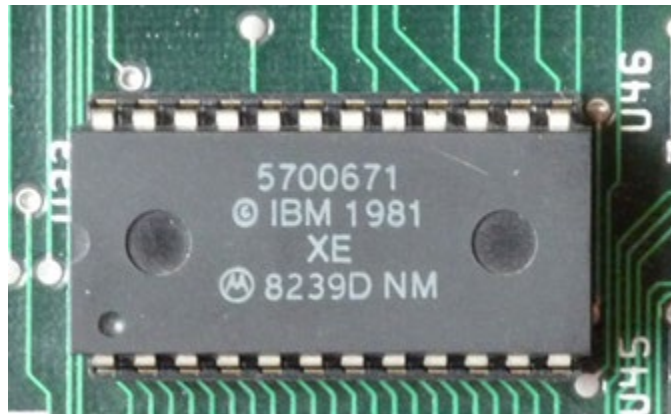
A ROM used in the 1981 IBM PC, depicted as installed in the motherboard 3
