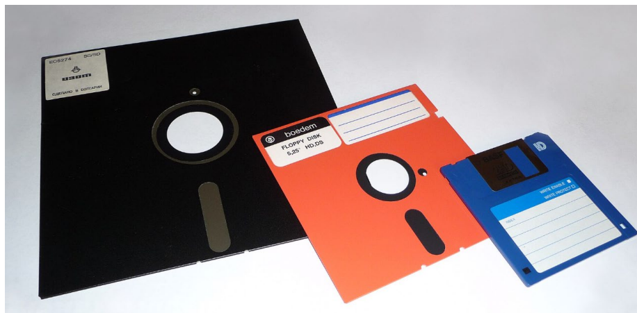
The three most common sizes of floppy disks in use around 2003. The 8” and 5.25” disks have a visible slot where the read/write head of the disk drive would access the disk; the 3.5” disk had a sliding metal cover over this slot to better protect the disk against contamination, scratches or other damage that could corrupt the data on the disk.
