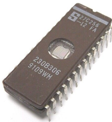
An EPROM with the erasure window visible as a circle in the top center of the chip.
