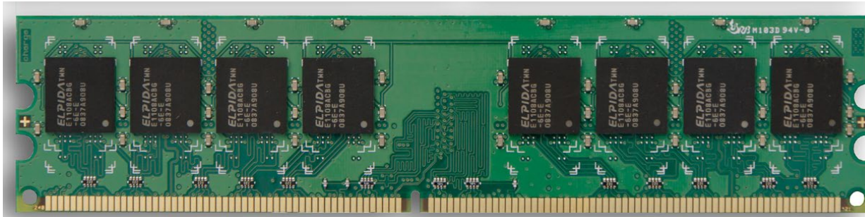
A 2GB DDR2 RAM module circa 2002. The RAM chips themselves are soldered into the module, but the module itself can be plugged into the motherboard (and removed) by a technician using proper precautions. The reverse side of this module also has RAM chips mounted; this is therefore called a DIMM (Dual Inline Memory Module).
