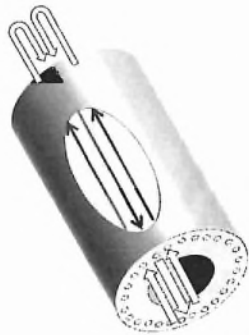
Figure 84. Peripherally drilled thermo roll with tri-pass II flow design.
