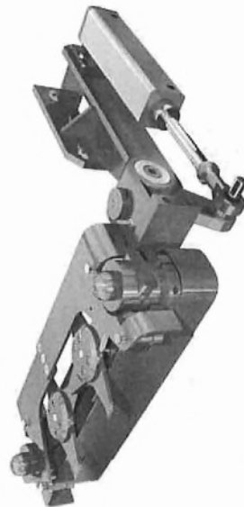
Figure 108. Rotary blade tail cut-off device 72 .
