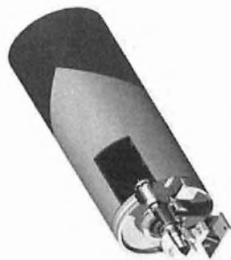
Figure 120. Typical construction of guide roll from composite material.
