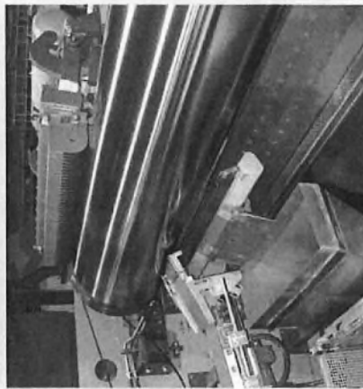
Figure 114. Disc roll-type pull-stack 78 .
