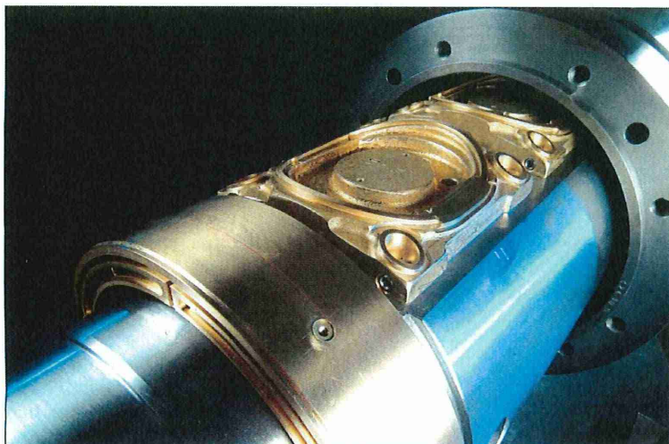
A PrimeRoll zone-controlled roll in the new BM2 calender
