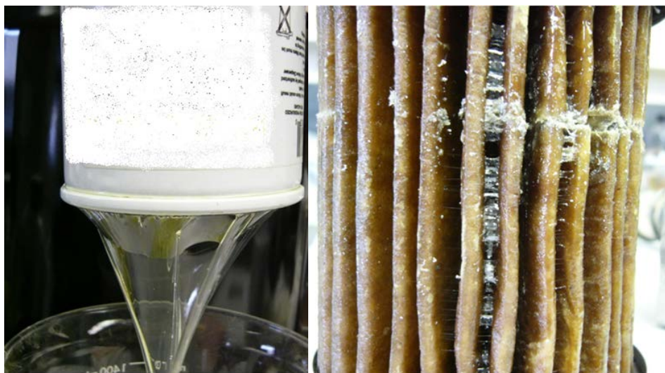
Figure 11: Unsheared DRA (left) and DRA blocking retail filter media (right) 7
