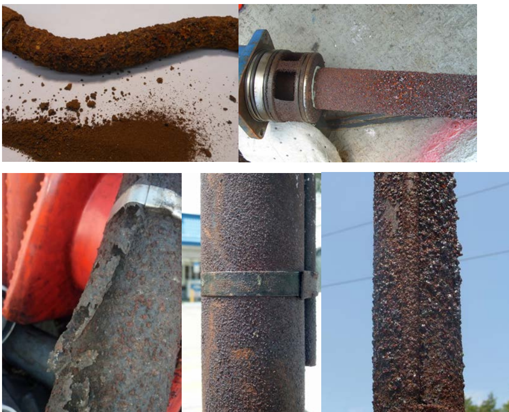
Figure 9: Microbially influenced corrosion of fuel storage and dispensing systems (Sources in clockwise order: Marathon Petroleum, Fuel Quality Services, Fuel Quality Services, Fuel Quality Services, Steel Tank Institute)
