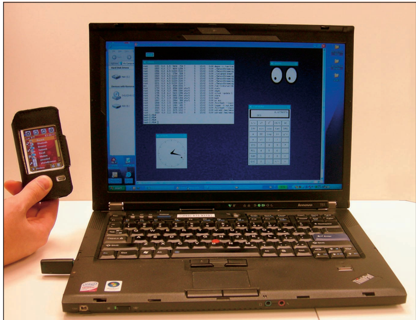
Figure 2. A Linux/XScale-based cell phone renders its desktop wirelessly to a nearby PC with a full-size display and keyboard, thus enabling effective user interaction.
