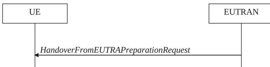
Figure 5.4.4.1-1: Handover from E-UTRA preparation request
