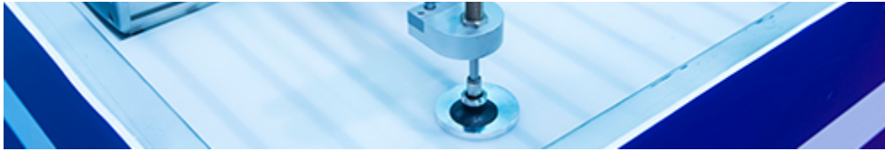
Figure 4: Double-acting cylinders can be used in a wide variety of ways, here we see a vacuum pick and place application that uses a pneumatic cylinder to move the position of the suction cup.
