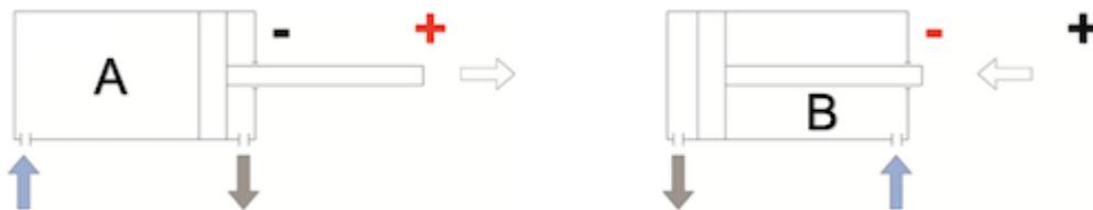
Figure 3: Double-acting cylinder working principle with air going in (blue arrow) and air coming out (grey arrow). The left image shows positive movement (A). The right image shows negative movement (B).
