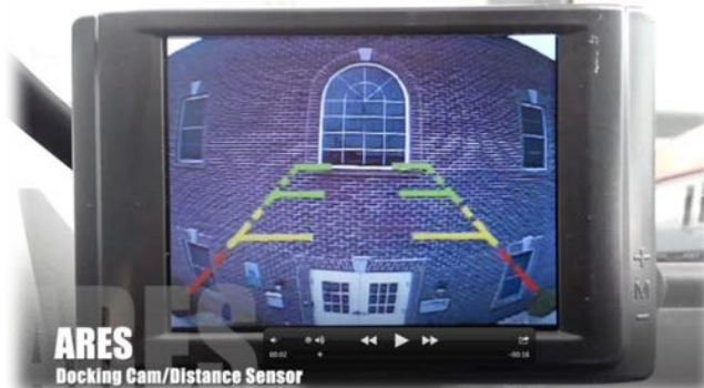
The ARES dash-mounted Monitor showing the driver the distance to target from the Breaching Platform Camera.
