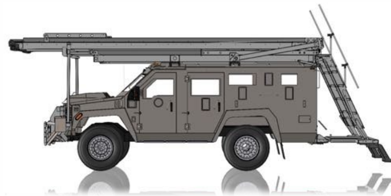
The ARES system on Lenco Bearcat, with Breaching Platform and Lifting Arms folded down for transport, and Rear Deployment Platform folded down for easy access to the ARES system from inside the vehicle crew area or on the ground.
