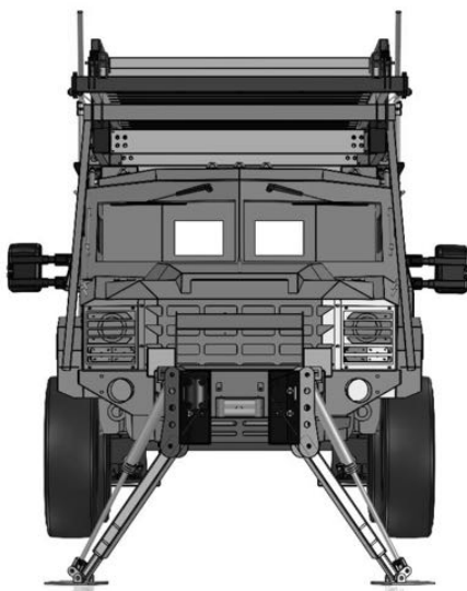
The ARES / Lenco Bearcat Fully-Armored Elevated Tactics Vehicle with integrated winch, and Front Hydraulic Stabilizers.
