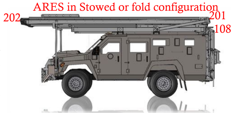
The ARES system on Lenco Bearcat, with Breaching Platform and Lifting Arms folded down, and Rear Deployment Platform folded up.
