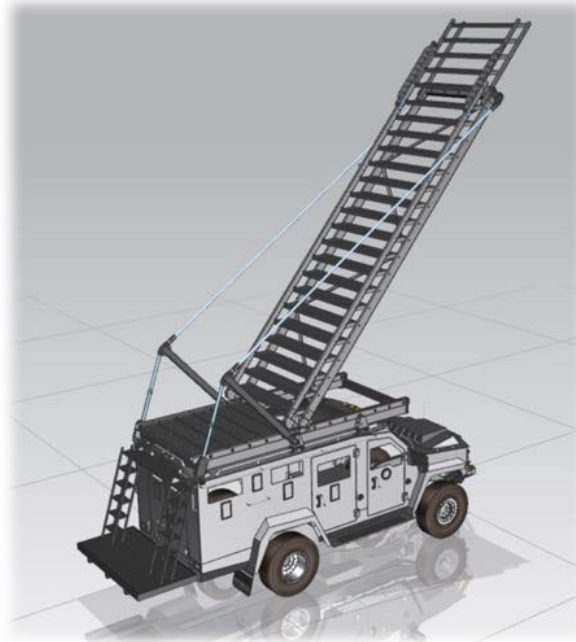
ARES Breaching Platform raised at the push-of-a-button as a stair extension up to 9 meters.
