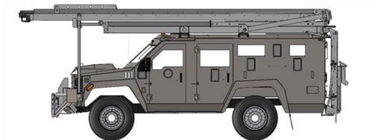
The Lenco Bearcat features circular gun ports on the front doors, and large, rectangular gun ports on the side doors, rear door, rear crew area, to allow for return of fire in every direction.
