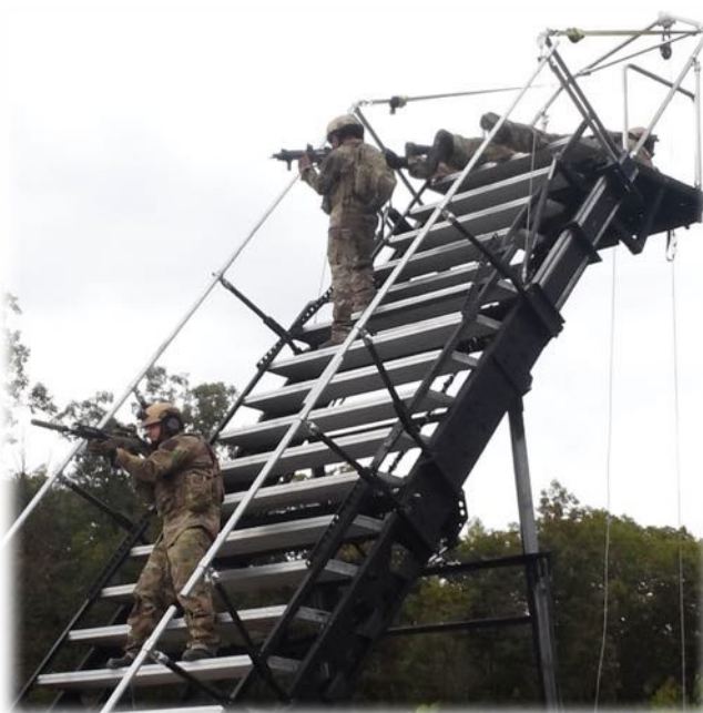
Operators easily stand on ARES' level steps, with a Sniper/Observer team on ARES' level Breaching Platform.
