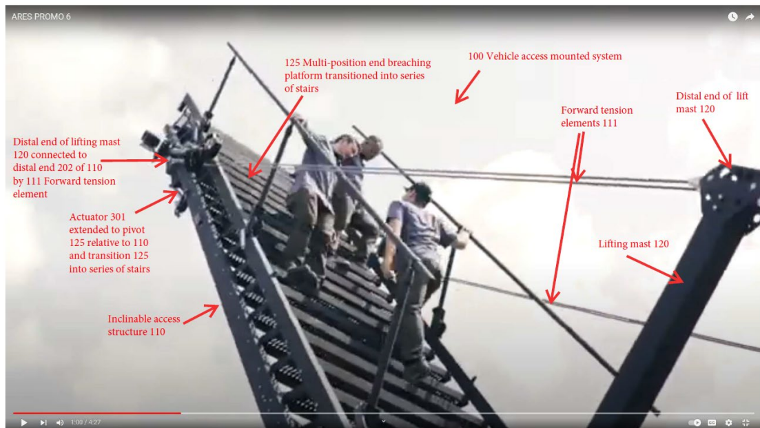
ARES 6 Video – annotated screenshot showing stairway elevated and extended, left side view. Ex. 1010, 4
