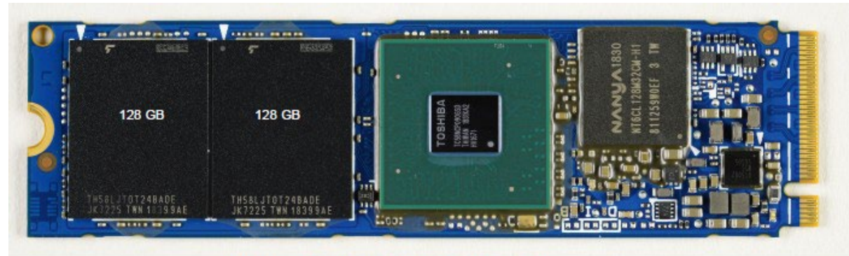
Toshiba KXG60ZNV256G SSD Package – Top
