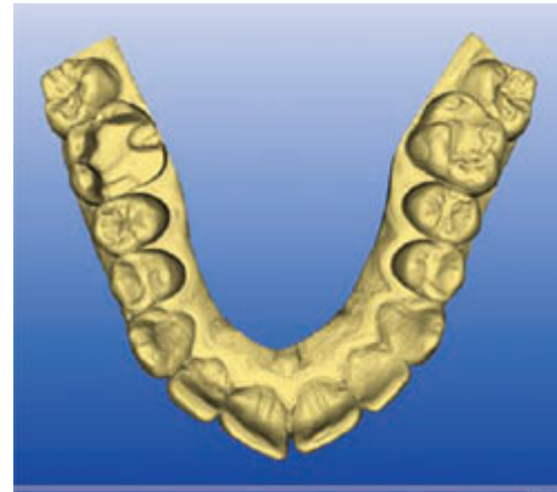
Figure 3 A screen shot of a full arch showing an onlay preparation on tooth No. 14. Userfriendly tools allow the refinement of a proposed virtual biogeneric restoration before milling.
