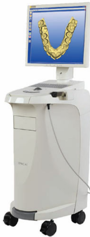
Figure 2 The CEREC AC BlueCam camera captures an image of teeth using a more precise, shorter wavelength blue light source via active triangulation sampling.
