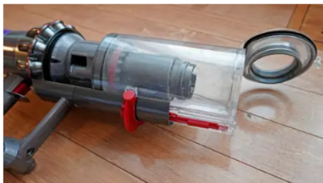
The dust bin also uses a redesigned emptying mechanism, but it might not actually be an improvement if you forget to lock it. Photo: Andrew Liszewski (Gizmodo)
