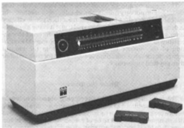
Fig 36. The Schleuniger or Heberlein tablet hardness tester shown with calibration blocks (courtesy, Vector).
