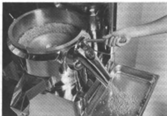
Fig 15. The inside of a QJ-400 Marumerizer (courtesy, Luwa).
