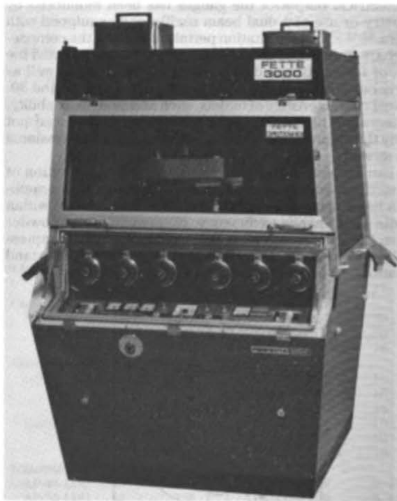
Fig 32. Fette Perfecta 3000 high-speed tablet press with pressing compartment completely sealed off from outside environment making cross contamination impossible (courtesy, Raymond Auto).
