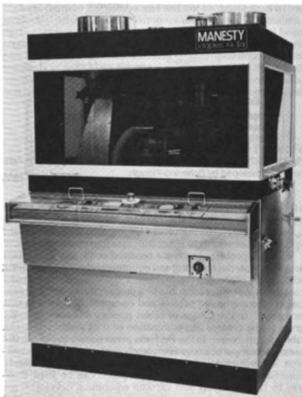
Fig 25. Rotapress Mark IIA: designed for improvements in sound reduction, operator safety, cleanliness and operational convenience; note the control panel on front of machine (courtesy, Thomas/Manesty).
