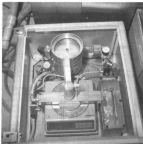
Fig 28. Direct weighing of tablets produced gives actual weight feedback for the controller of the Courtney R-100 (seen in the bottom left of Fig 27).
