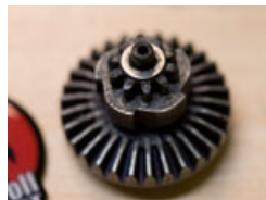
The bevel gear has five anti-reversal latch teeth.
