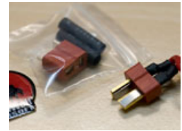
The Deepfire M4 is wired with a deans connector and includes a spare set for your charger.
