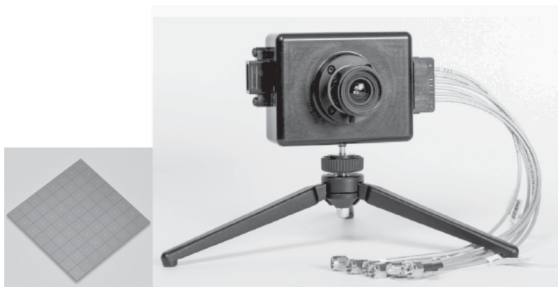
Figure 6-25 (left) A commercial 8x8 channels SiPM of 3 \times 3 \text{ mm}^2 channel area with 3584 individual SPADs, 50\text{-}\mu\text{m} pitch, and 0.74 fill factor (courtesy of Hamamatsu); (right) a turnkey module with an SPAD array of 64 \times 32 smart pixels comprising SPAD, front-end and processing circuits, with a 9.6 \times 4.8\text{-mm}^2 sensitive area, and 96-kf/s frame rate (courtesy of Micro Photon Devices, Bolzano).
