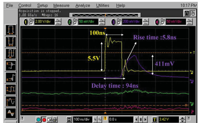
Fig. 8. Voltage waveform driving the LD (upper trace) and output voltage waveforms from SiPM devices in the array (all other traces) for the single-target rangefinding experiment. The light reflected from the target was projected on SiPM 6, which produced the highest output pulse voltage.
