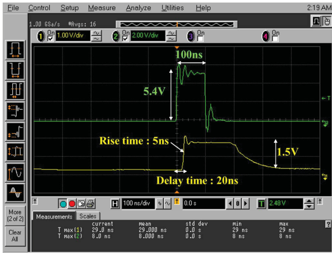
Fig. 6. Voltage waveform that drives the LD (upper trace) and output voltage waveform from the SiPM that picks up the light pulse reflected from the target.
