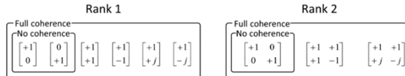
FIG. 11.10 Uplink codebooks for the case of two antenna ports.
