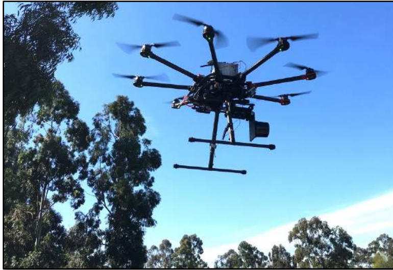
Figure 11. Drone with Side-Mounted Sensor
