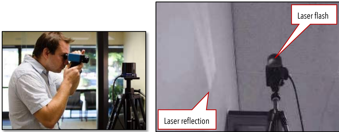
Figure 42. View Sensor through IR Scope (left) to See Sensor Flash+Reflection (right)
