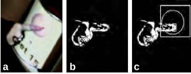
Figure 6. Detecting a touch: a) camera view of an interaction with a bucket; b) image difference data; c) overlay of search region (square), button active area (circle), and the fingertip template shown at the pointing location.
