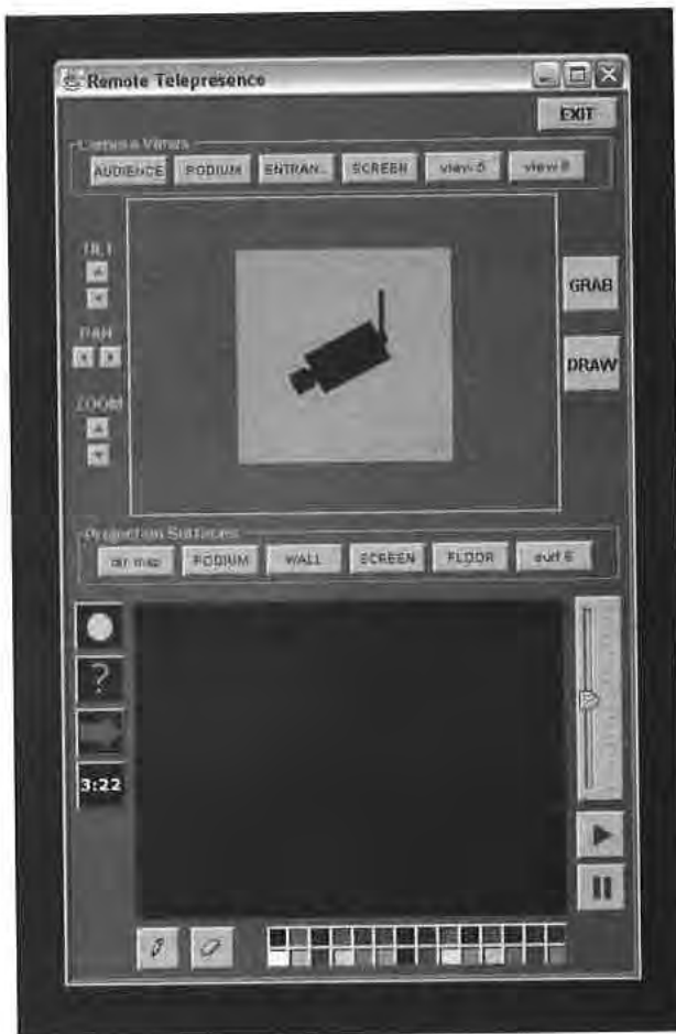
Figure 2. Example of control interface for a remote session chair using a projector-camera system to communicate with local conference participants.
