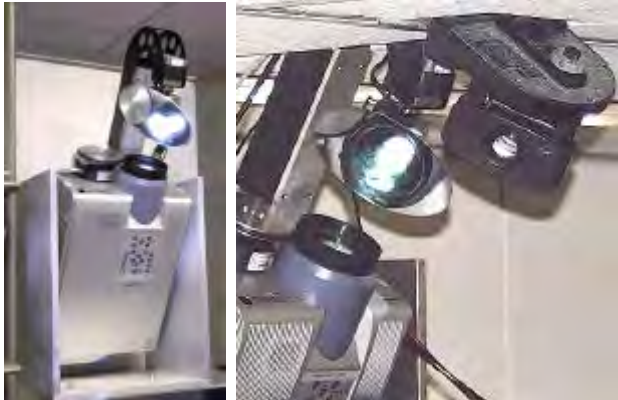
Figure 3. Prototype of the ED-projector: a) ED-projector without the camera mounted; b) a detail of a complete prototype, including the pan/tilt camera.
