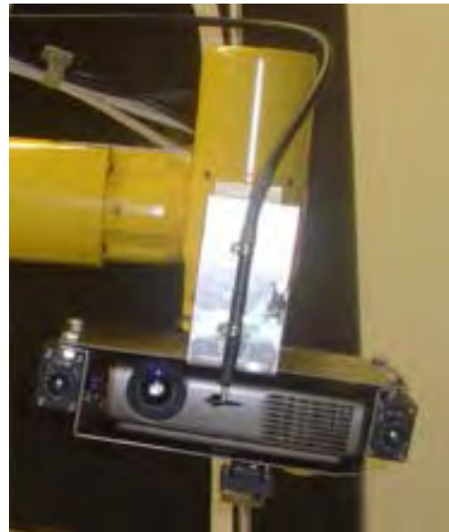
Fig. 2 Projection-vision system mounted to hand of the robot.
