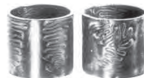
Figure 10-120 Two molded bushings showing poor surface finishing
