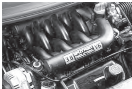
Figure 10-30 Lost core thermoplastic V-6 intake manifold (Courtesy: Ford)
