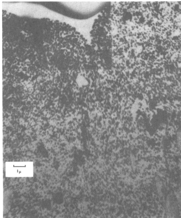
Fig. 6-46 A 5- \mu -deep SMA weld line from a sample molded at 470°F (243°C). Rubber particles are elongated parallel to the weld line.
