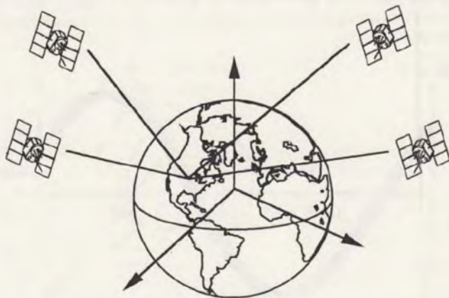
Figure 3.14 ECEF Cartesian coordinate system for GPS.
