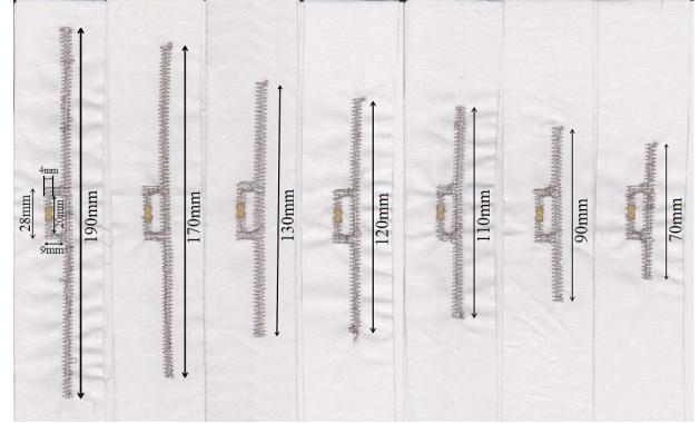
Figure 5. Sewed antennas with the same T-match geometry as before, but with different lengths.
