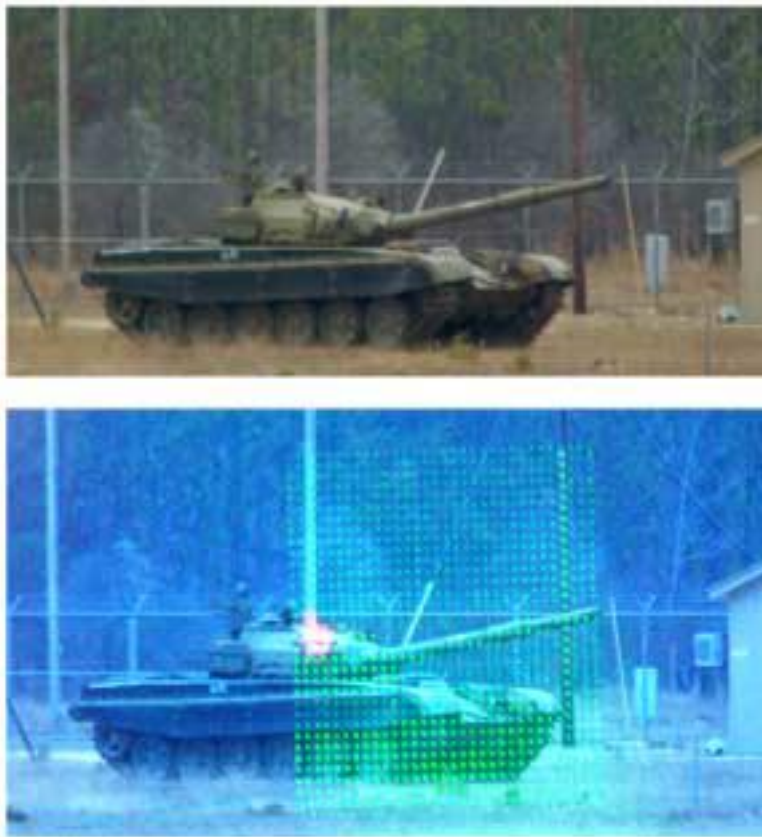
Figure 8: Two photographs of a tank vehicle. The upper image is a visible color photograph that was taken while the laser was off. The bottom photograph was set with a long exposure and green-enhanced to show an image of the 532 nm 32x32 laser spot pattern as it was backscattered from the target scene.
