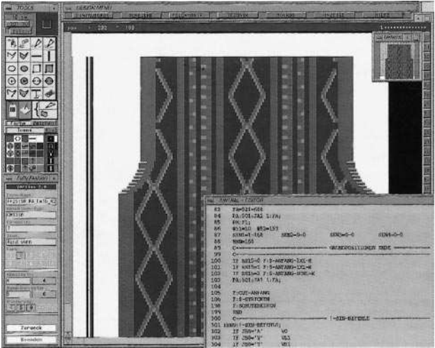
Fig. 12.6 The FF programme inserts the control columns and, using the existing jacquard, generates the Sintral programme, which contains all the necessary data for machine control [Stoll].
